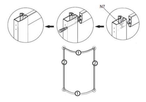
Place the front glass panels (3) into the side profiles, ensuring these are fully inserted push in the glass gasket (L3) between the profile and the glass and push in fully to secure the glass, cut down to suit.
