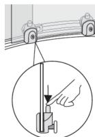
Once the doors are installed, the door stops (J2) need to be fitted. Secure these to the frame using the screws provided (N5) Fit the magnetic door seals (L1) to the edge of the door. The door seals (L2B) should be fitted to the doors, as shown below with the fin facing outward from the tray.
